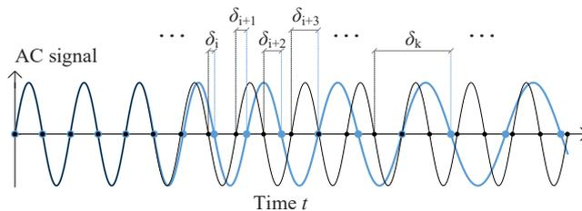
Fig. 6. Zero-crossing detection process
