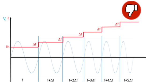
Fig. 11. Graph of a non-“stepless” (continuous) frequency ramp. This ramp is not allowed. Depending on the size of steps and relay algorithms, different results may be obtained for the same relay.
