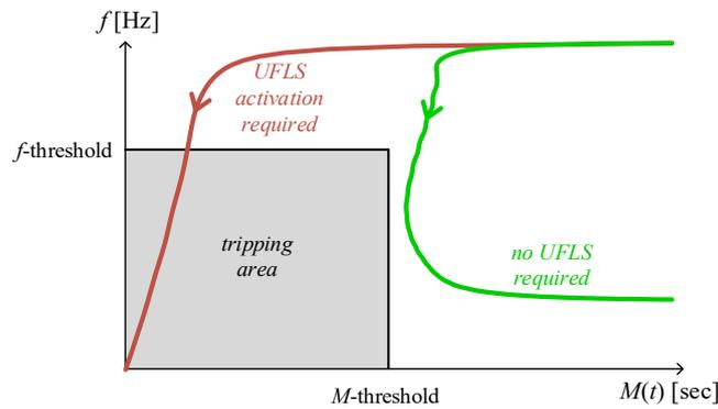
Fig. 8. Using frequency-stability margin  $M(t)$  for setting the UFLS tripping criteria
