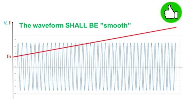
Fig. 10. Graph of the “stepless” (continuous) frequency ramp used to assess ROCOF and frequency relay performances
