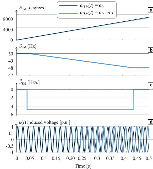
Fig. 5. Rotor angle (a), rotor speed (b), rotor acceleration (c) and generated induces voltage (d) during constant angular deceleration
