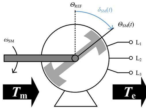
Fig. 3. A conceptual representation of a synchronous machine
