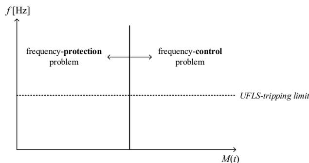
Fig. 7. Frequency-stability margin  $M(t)$  might help to differentiate between the frequency-control and frequency-protection problems
