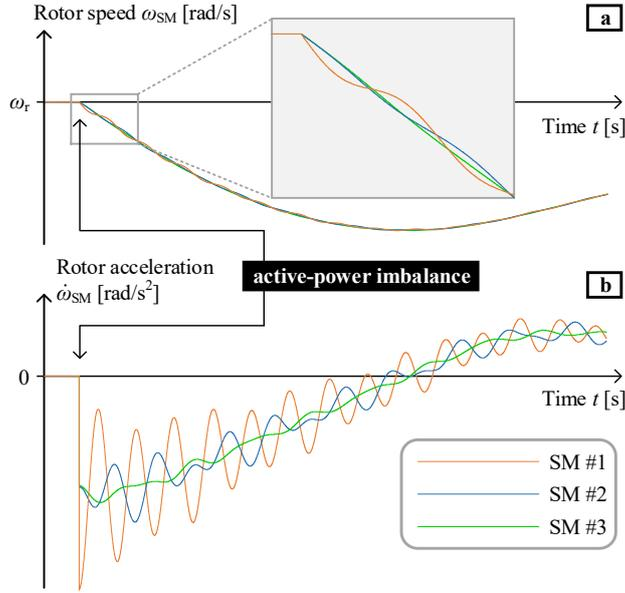
Fig. 4. Rotor speed (a) and acceleration (b) of different SMs in the network following an occurrence of an active-power imbalance
