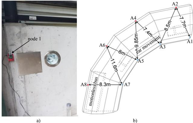
Fig. 2. Measurement setup; a) photo at the location and b) Tx/Rx positions with moving car and motionless bus
