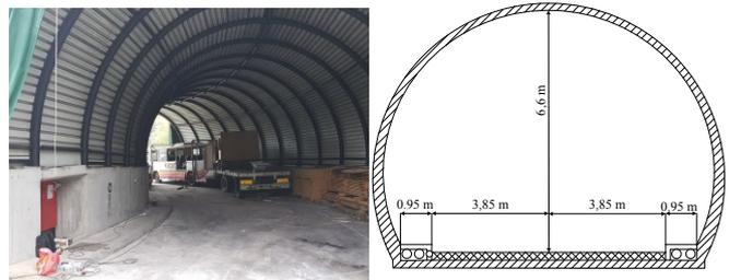
Fig. 1. Tunnel construction and cross-section dimensions
